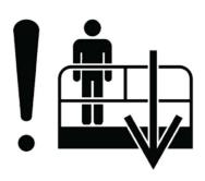
A decal may be positioned directly above or in the vicinity to identify the location of the emergency/auxiliary lowering controls
